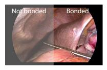
FSN's optical bonding process (right) improves contrast ratio and brightness, and increases humidity resistance and breakage resistance.
